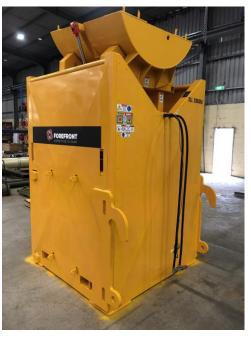
Forefront Services was engaged to design and manufacture a hydraulically controlled lifting rig for installing vent fans to the roof of roadway tunnels. The client required the design to be simple with no complex connections and the unit needed to be robust enough to cope with the aggressive tunnel environment.
